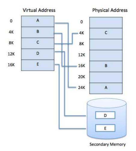
Virtual memory is commonly implemented by demand paging. It can also be implemented in a segmentation system. Demand segmentation can also be used to provide virtual memory.
